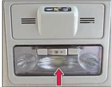
Front roof lamp
