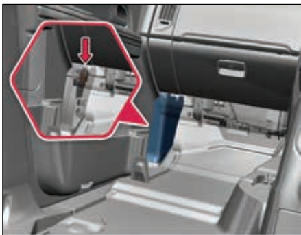
Inertia switch location
