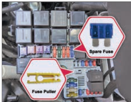
Engine compartment fuse box
